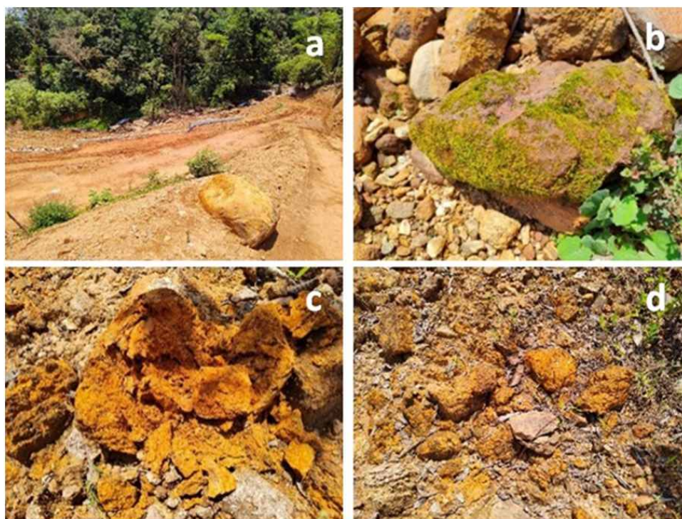
Fig. 3. Fresh rock (a), corestone (b), decomposed granite (c) and fine-grained saprolite (d).
